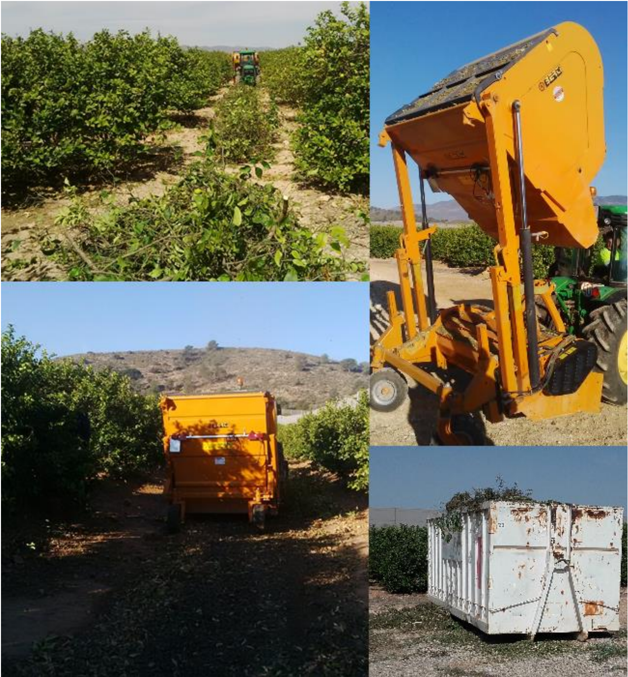
Figure 4 – Shredding tool with tipper integrated (Source: Life Ecocitric)
