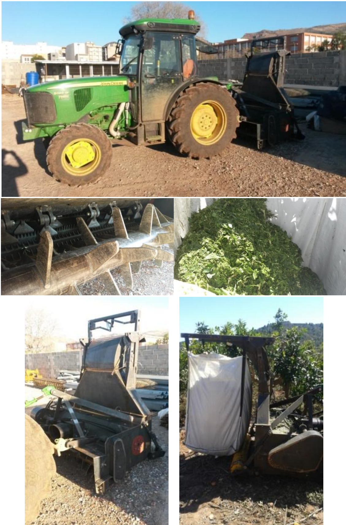
Figure 3 - Tractor with shredding equipment with direct loading in big-bags (Source: Life Ecocitric).
