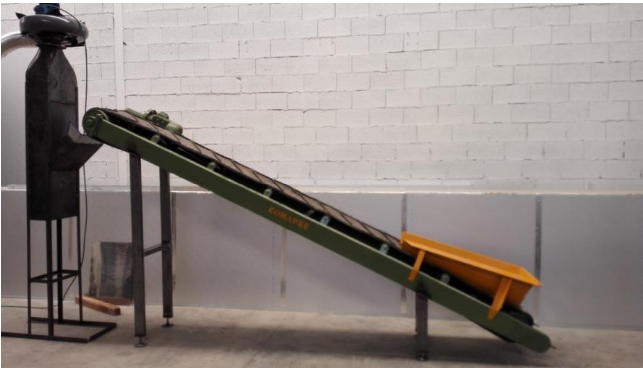
Figure 10 - Separation tower and collection system of raw material
